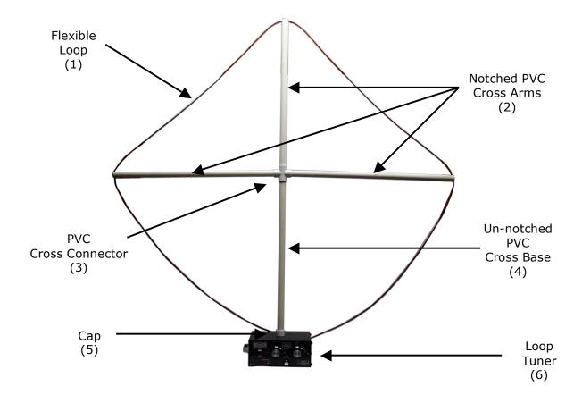
Figure 1: PVC Cross Mount Loop Assembly
